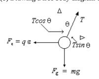
Resolving *T* into horizontal and vertical components:  $T \cos \theta = mg$
